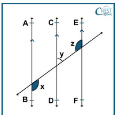
$$\angle x = \angle z \text{ (alternate angles, } AB \parallel EF\text{)}$$
